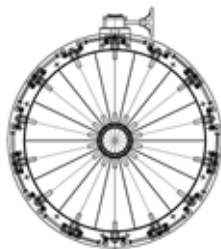
CVC-01 - Inlet Vane Control Damper
